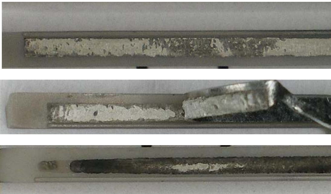
Figures 5: Parts are arranged by darkest to lightest (zirconia tint) from top to bottom. The middle part is shown midway through the peeling process and BFM can be observed on both the zirconia and the stainless surfaces such that the weak point is the alloy itself (as desired). The darker residue in the bottom part (with the lighter zirconia) shows only a small amount of BFM residue. The darker residue may be the result of an oxide and/or Ti intermetallic formation caused by poor contact of the BFM preform with the zirconia substrate.
