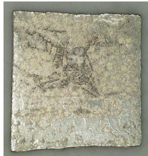
Figure 1: Square of active braze foil fused onto alumina at approximately 940°C in partial pressure inert atmosphere
